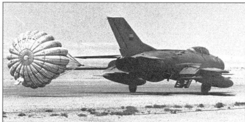
One of the UARAF's ex-Iraqi MiG-19Ss lands with its braking parachute deployed on either 20 July or 11 August 1965 (EAF)
